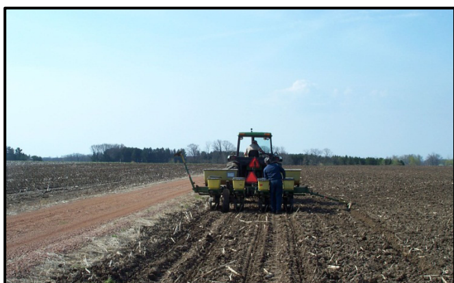
Figure 2. Adaptation of a traditional row (corn or soybean) planter for establishment of eastern gamagrass.
